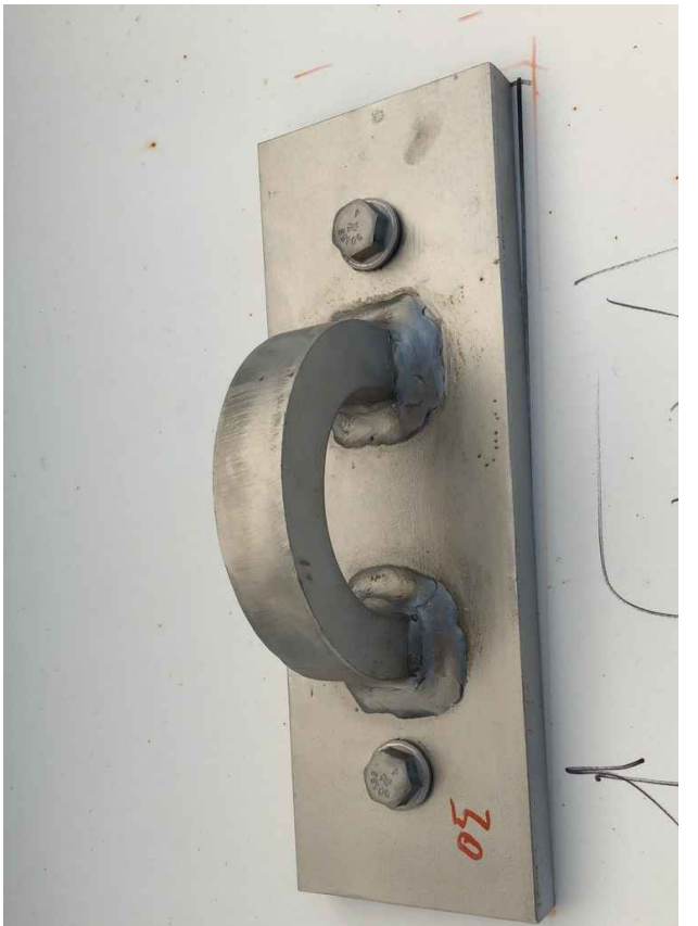
South Hampton - Roof Anchor #30 - pretest.
