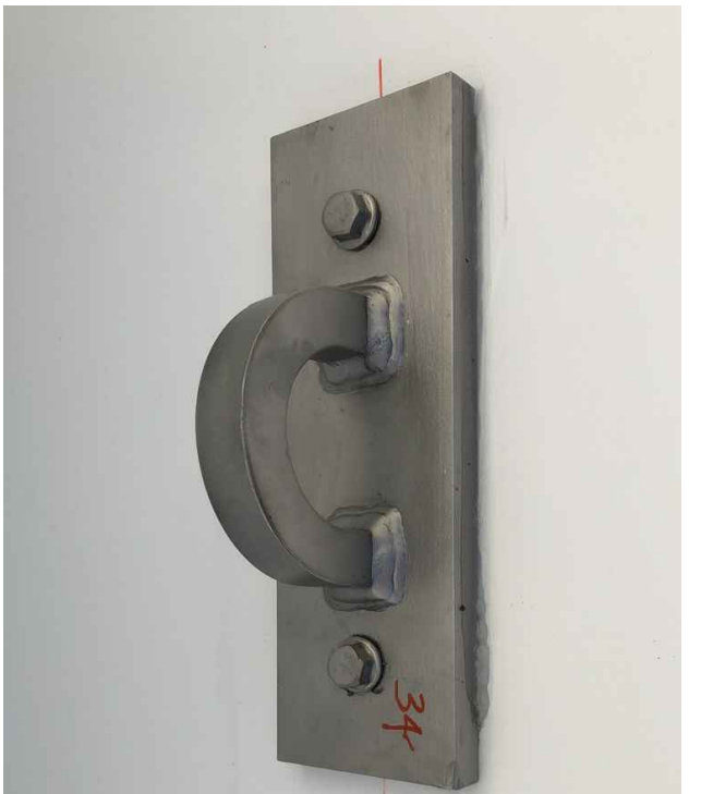
South Hampton - Roof Anchor #34 - pretest.
